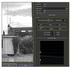
Manual mode provides more control than Auto. For example, the user may only want to run with an upper threshold (trigger on brighter, not darker).
