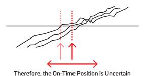
Generator and camera timings can be inaccurate relative to each other depending on factors such as temperature, age and manufacturers' tolerance.
