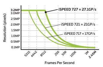
The 27.1 GPixels/s raw throughput rate is the fastest in the industry. No spatial or temporal interpolation. Raw speed, the 168ns shutter time is also among the fastest. We even optimized the 13.5 µm pixel size for the proper balance between high-resolution (for image clarity) and exceptional light sensitivity normally found only with larger pixels.
